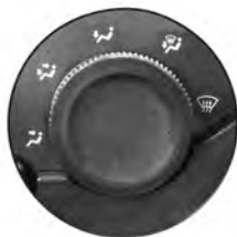
Air distribution control
