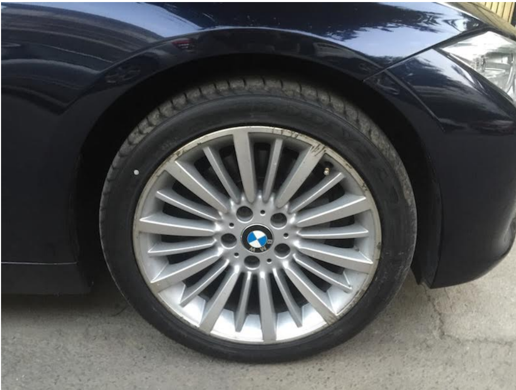
No attention to detail for tire install, notice that white dot it should be opposite side of the valve (it denotes the lightest part of the tire)
