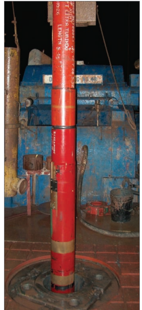
Figures 5 (above) and 6 (right): The hydraulically opened downhole deployment tool was evaluated in the last well for suitability as a barrier and to eliminate the need for a hydraulic workover unit. Table 1 (below) summarizes run conditions for the mechanically operated downhole isolation valve (PWI-1, UBD Oil-1, UBD Oil-2) and the hydraulic downhole isolation tool (UBD Oil-3).
