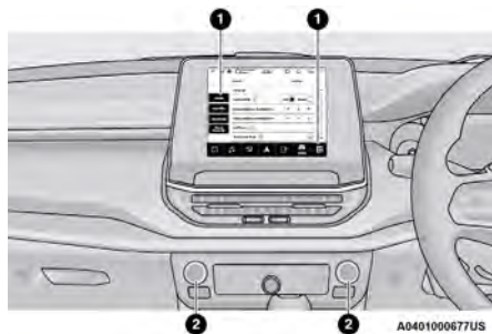
Uconnect 5 With 8.4-inch Display Buttons On The Faceplate And Buttons On The Touchscreen
