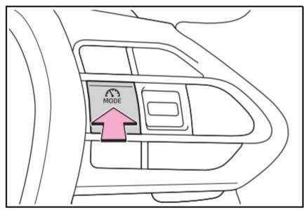
Using the accelerator pedal, accelerate to the desired vehicle speed (approximately 30 km/h [20 mph] or more), and press the driving assist switch to set the set vehicle speed.
