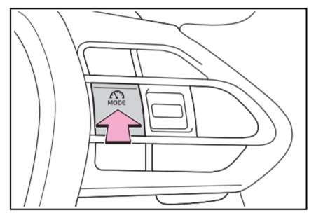
2. Using the accelerator pedal, accelerate or decelerate to the desired vehicle speed (approximately 30 km/h [20 mph] or more), and press the driving assist switch to set the set vehicle speed.
