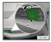
Screw in the towing lug by turning to the left -arrow- with the hand up to the stop.
