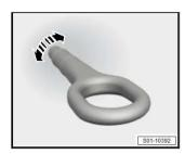
Tighten the towing lug with the wheel bolt key (push the key through the lug).
