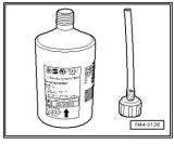
In this example, the best-before date 05/2003 has expired and the bottle must then be replaced.
