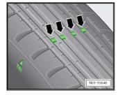
If the tyre tread depth is close to the legal minimum, the customer should be informed of the necessary tyre change.
