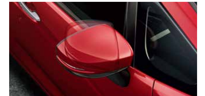
Electric Mirror with Turn Indicator
