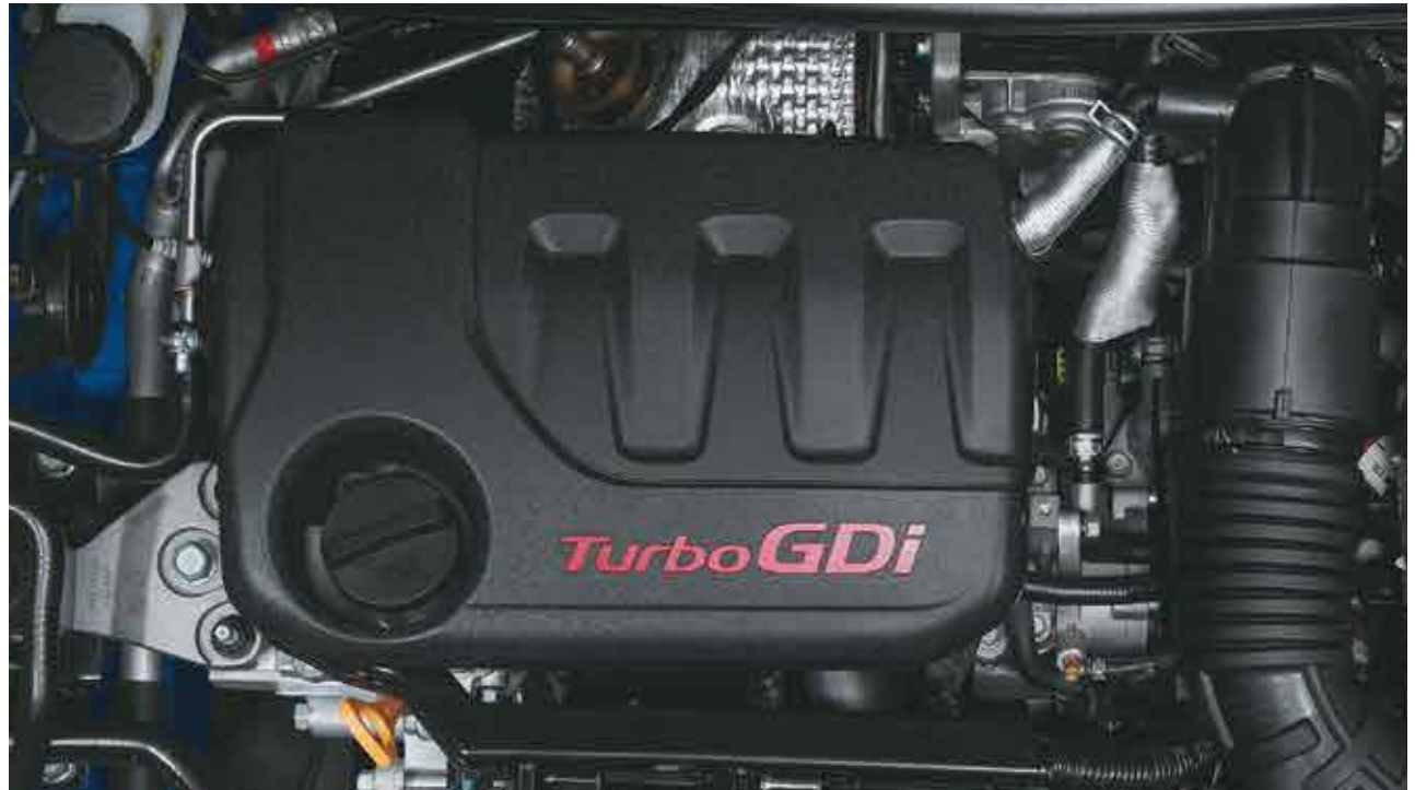
1.0 I Turbo GDi petrol engine with max. power of 88.3 kW (120 PS) / 6 000 r/min
