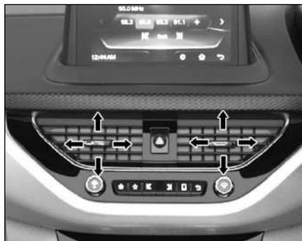
Centre Air Vents (Front)
