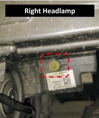
Do both headlamp adjustment at same height and check for horizontal leveling by doing a small drive in nearby streets. This is to ensure that oncoming vehicles are not affected by this light output when leveler is kept in position ZERO (highest setting).
