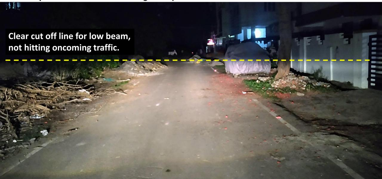
**END RESULT:** Low Beam + High Beam + fog lamps – light spread after realignment – much wider than stock. Road is lighted up on both sides uniformly until the edge of the road and beam intensity remains the same. This light output is on a dark road.
