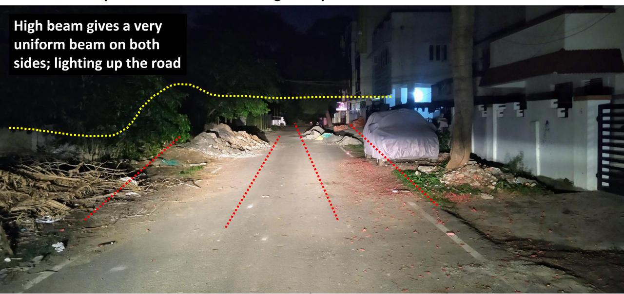
**END RESULT:** Low Beam + + fog lamps – light spread after realignment – much wider than stock. Road is lighted up on both sides uniformly until the edge of the road and beam intensity remains the same. This light output is on a partially lit road.
