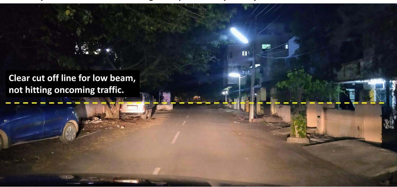
**END RESULT:** Low Beam + High Beam + fog lamps – light spread after realignment – much wider than stock. Road is lighted up on both sides uniformly until the edge of the road and beam intensity remains the same. This light output is on a partially lit road.
