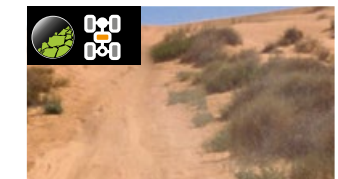
4LLC (4WD Low Range with locked centre differential) For steep hills, sand, deep snow, etc.*
