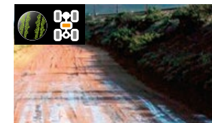
4HLC (4WD High Range with locked centre differential) For rugged terrain with low-grip surfaces.*
