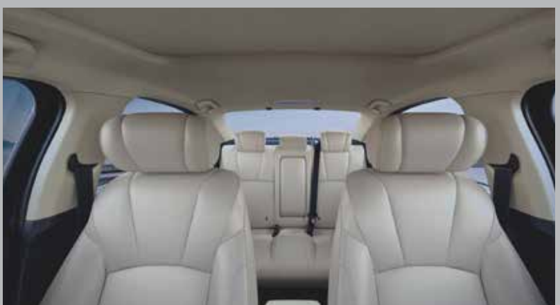
ALL SEATS HEAD RESTRAINTS WITH 3-POINT ELR SEATBELTS
