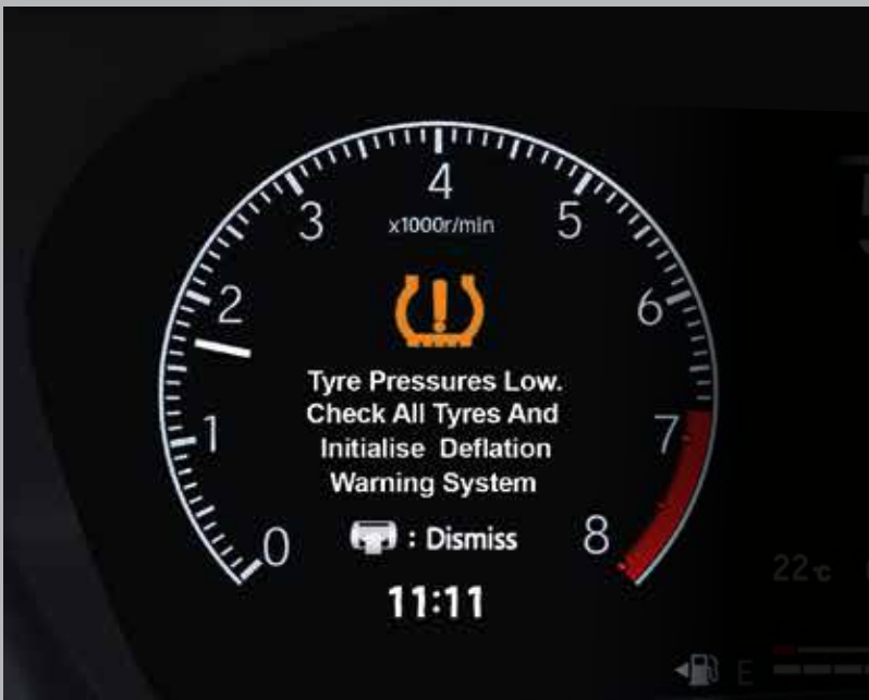
TYRE PRESSURE MONITORING SYSTEM (DEFLATION WARNING SYSTEM)
