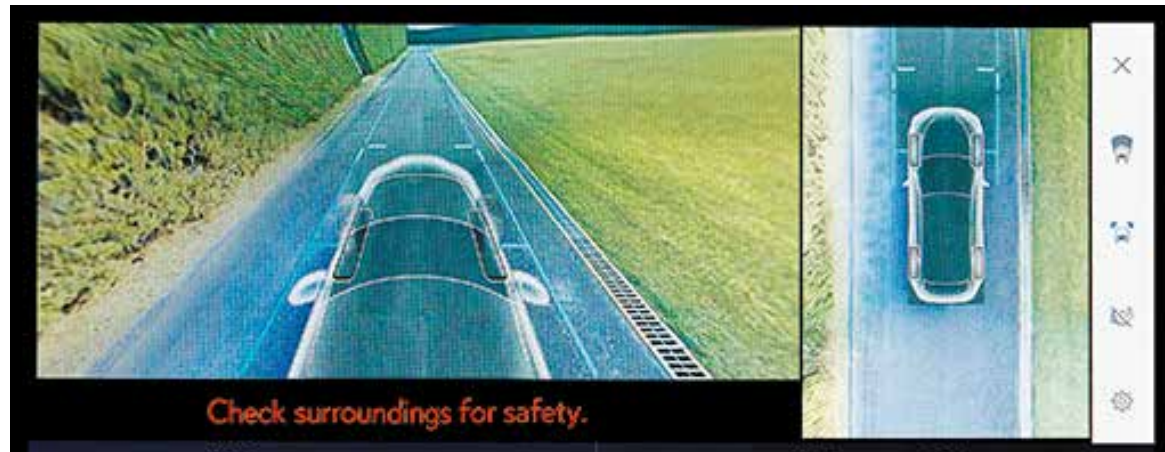
Panoramic View and Side Clearance View
