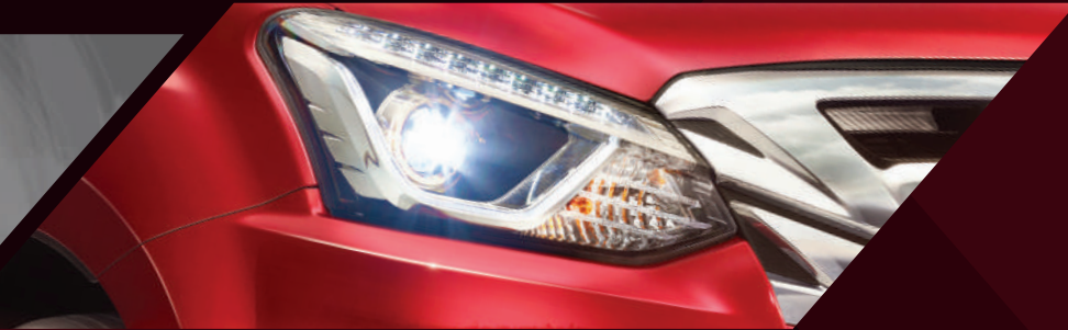
Bi-LED Auto -levelling Headlamps with DRL
