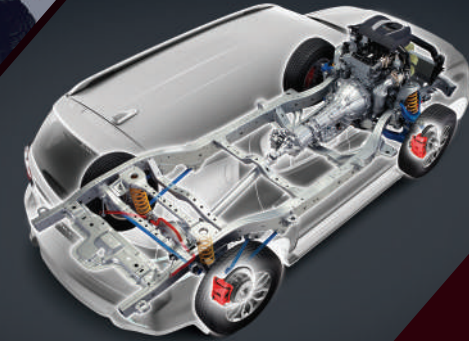
Heavy - duty Ladder Construction Chassis
