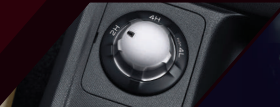
'Shift-on-the-fly' 4x4 Select Dial for Fingertip Terrain Control
