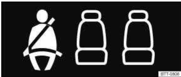
Fig. 28 On the instrument cluster display: seat belt status for the rear seats.
