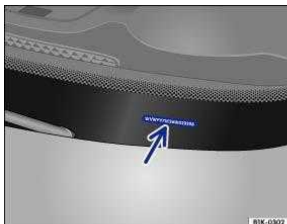
Fig. 213 : vehicle data sticker: the example shows a vehicle with engine code CPTA (3) : type plate.
