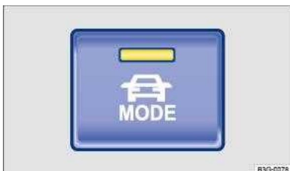
Fig. 110 In the lower section of the centre console: driving profile selection button.
