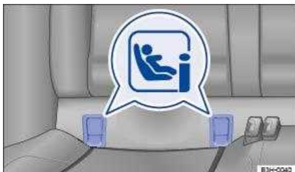
Fig. 46 Markings identifying the ISOFIX anchor points for child seats.
