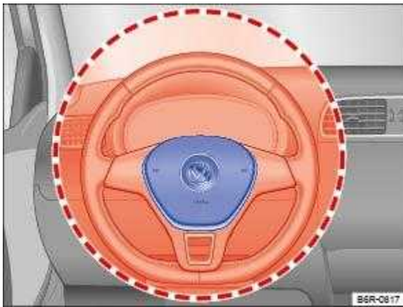
Fig. 40 Location and deployment zone of the driver front airbag.
