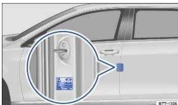
Fig. 195 On the driver door pillar: tyre pressure sticker (alternatively on the inside of the tank flap).
