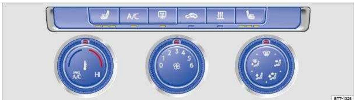
Fig. 91 In the upper part of the centre console: air conditioning block for the manual air conditioning system and heating and fresh air system.
