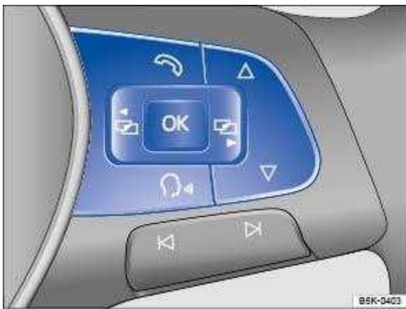
Fig. 21 Right-hand side of the multifunction steering wheel: controls for using the menus and information displays in the instrument cluster.
