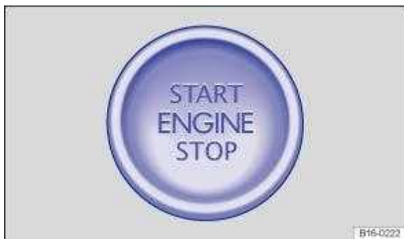
Fig. 100 In the lower section of the centre console: starter button for starting the engine.
