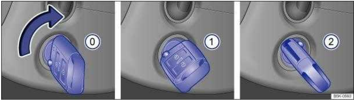
Fig. 99 To the right of the steering wheel: positions of the vehicle key in the ignition lock.
