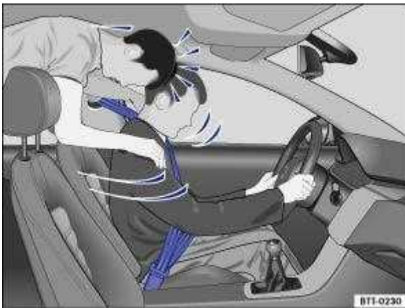
Fig. 32 The unbelted rear passenger is thrown forward and strikes the belted driver.
