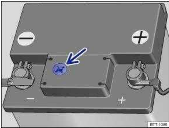
Fig. 192 Battery window on the top of the 12-volt vehicle battery (illustration).
