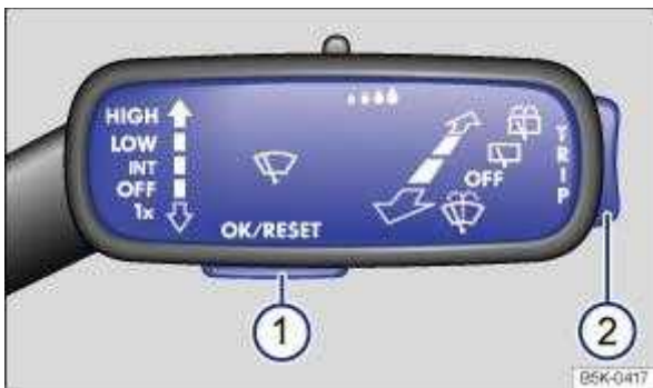
Fig. 20 On the right of the steering column: buttons on the wiper lever (illustration).
