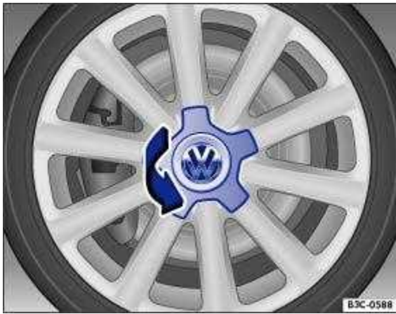
Fig. 200 Removing the centre wheel trim by turning.
