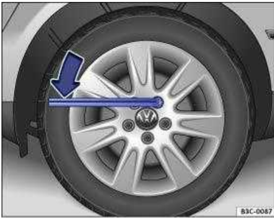
Fig. 203 Changing a wheel: loosening the wheel bolts.
