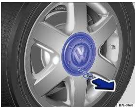
Fig. 199 Removing the centre wheel trim by pulling.
