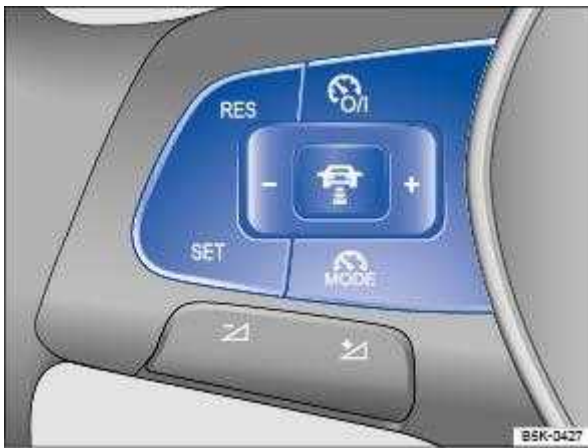
Fig. 117 Left-hand side of the multifunction steering wheel: buttons for operating the speed limiter.
