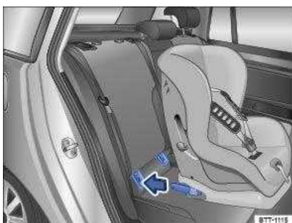
Fig. 47 Illustration: fitting an ISOFIX child seat with attachment arms.
