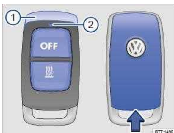
Fig. 93 Auxiliary heater: remote control (left) with battery compartment (right).
