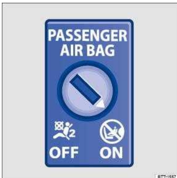
Fig. 42 In the dash panel on the front passenger side: key switch for disabling and enabling the front airbag on the front passenger side.
