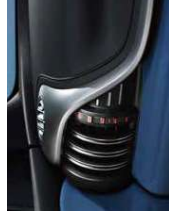
Dumbbell-style Air Conditioning Vents
