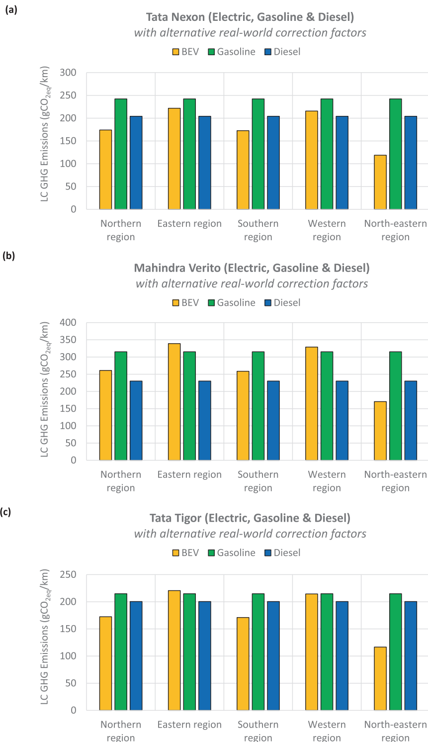
Fig. 9 The effects of adopting an alternative set of real-world correction factors on the life cycle (LC) GHG emissions of electric, gasoline, and diesel vehicles. Compared to the NEDC, the electric range of a battery-electric vehicle (BEV) is reduced by 30%, while the fuel consumption of combustion engine vehicles increased by 34% 76 . A total vehicle lifetime distance of 200,000 km was assumed for (a) Tata Nexon, (b) Mahindra Verito, and (c) Tata Tigor.
