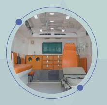
MiTR Ambulance comes with customisable interiors and ample storage space for equipment and consumables. It has a reinforced sidewall for mounting critical-care equipment like defibrillators, suction pumps, and more. Apart from this, it also has an auto-loading, foldable stretcher cum
