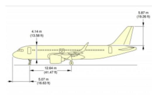
There is a clearance of approx 1 meter of engines of an airbus 320 from ground , so if landing gears are down there is no way engines can hit the runway. Once gears are retracted only then engines will touch the ground . So at least this thing is sure that aircrfat gears were not lowered (intentionally or any malfunction) yet to be determined . Another data shown below also reveals that the aircraft came down very low and then again climbed
